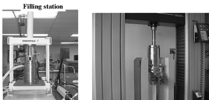
Figure 8. Off-line version of the adjustable gap slit rheometer and filling station [14].
